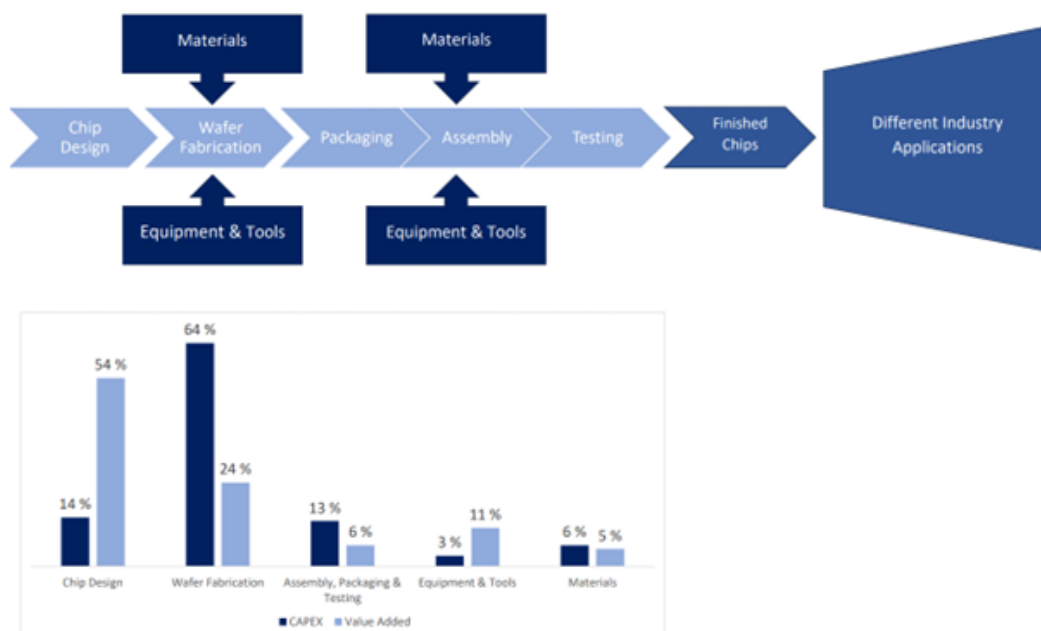
Figure 1: Main value-adding steps of the semiconductor supply chain 1
